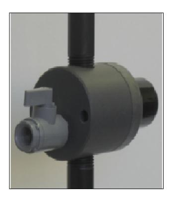
**Griffco** diaphragm backpressure valves are designed to enhance the performance of chemical feed systems. The addition of a priming valve to the backpressure valve enables the manual priming of the chemical feed pump. Available in PVC, PP, PVDF and 316 SS. Others available on request.
