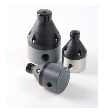
**Griffco** high flow diaphragm back pressure valves are designed to enhance the performance of higher flow, continuous feed pumps that require a constant head pressure, while also acting as an anti-syphon valve. Larger orifice sizes make the valve ideal for use with higher viscosity fluids. Wetted materials include: **PVC, CPVC, PP, PVDF, PTFE, 316 SS, A 20 and Hast. C.** Available in DN15, DN20, DN25.
