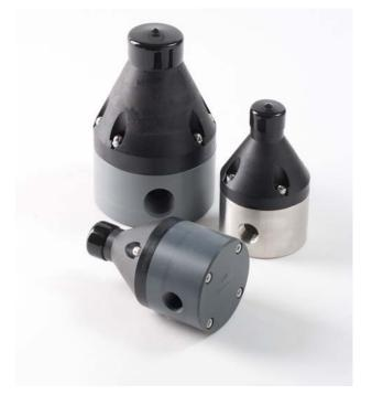
Griffco high flow diaphragm pressure relief valves are designed to protect chemical transfer systems from over pressure damage caused by defective equipment or a blockage in the chemical line. Large orifice sizes facilitate high flows and high viscosity. Wetted materials include PVC, CPVC, PP, PVDF, PTFE, 316SS, A20 and Hast. C. Available sizes: DN 15, DN 20 and DN25.
