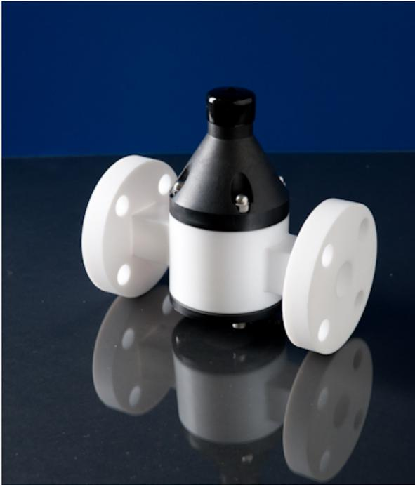
**Griffco G-Series** diaphragm back pressure valves are designed to enhance the performance of chemical feed systems by applying a continuous back pressure to the chemical feed pump, while also acting as an anti-syphon valve. Robust construction ensures reliability in the rigorous service of sulphuric acid for both municipal and industrial applications. Wetted materials are: **PTFE**. Available sizes: DN15 – DN25.
